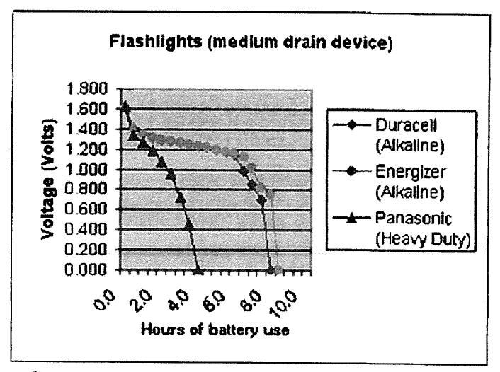
The heavy duty battery by Panasonic holds less Voltage Over time than the alkaline Duracell and Energizer batteries. The Panasonic hattery lasted approximately 5 hours. The two alkaline batteries, Duracell and Energizer lasted approximately 8.5 and 9 hours respectively. Therefore, the flashlights with alkaline batteries can be used almost twice as long as a flashlight with a heavy duty battery.
